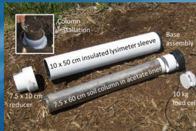
An Automated Microlysimeter Design for Soil Evaporation Monitoring.
